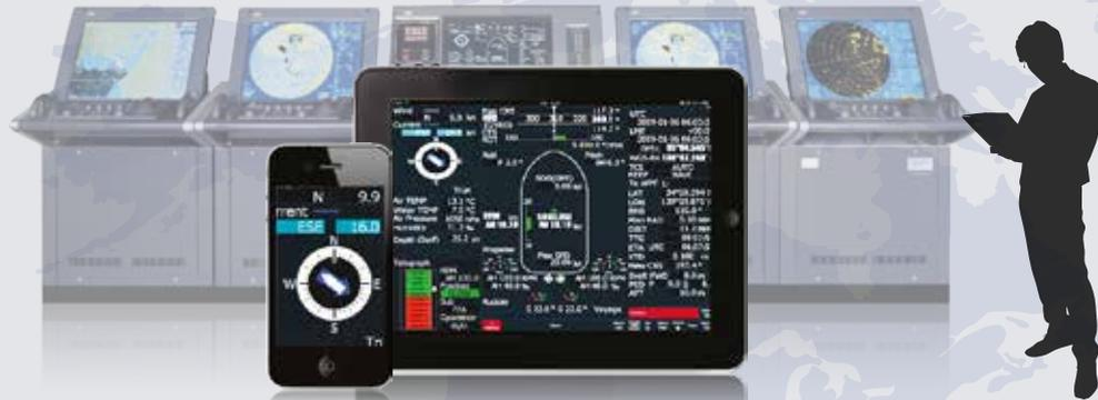
myView delivers the bridge's navigation and security situations in a type of streaming videos to your smart devices, tablets and desktop through ship's wire or wireless network. With this feature, you can select and monitor the equipment in your bridge such as Radar, ECDIS, Conning and CCTV on your mobile anywhere on board ship, just like you work on the equipment.
