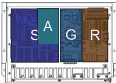
Interface circuit arrangement in NQE-1143 Junction Box
